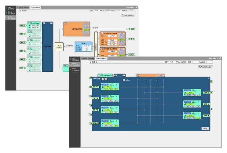
The graphical configuration interface of the Ethernet switch part allows the management of IP flows with a principle similar to video matrix, this allows a simplification in configuration and management of the part of networking.
