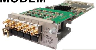
The EK-UNM/4 board is a digital single carrier modem with Adaptive Code Modulation that allows the conversion between the Base Band streams in a intermediate frequency and vice-versa. The card is designed to be inserted in all the versions of the EK-MFR/x frames that allow a completely management and configuration of it.
