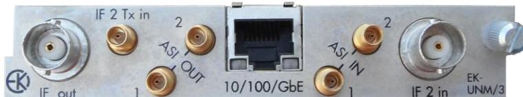
The revolutionary feature applied to this board is the possibility to use at the same time both **GbE** and **TS ASI** interfaces selecting the data rate preferred for each IN/OUT so it is possible combine ASI and IP technology in broadcasting activities and to prepare a complete migration to IP.
