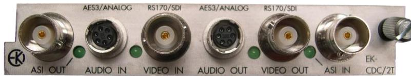
The board EK-CDC/2T allows to code and decode a video signal plus two audio channels in digital form according to specific MPEG-2 (Main profile@ Main level 4:2:0).
